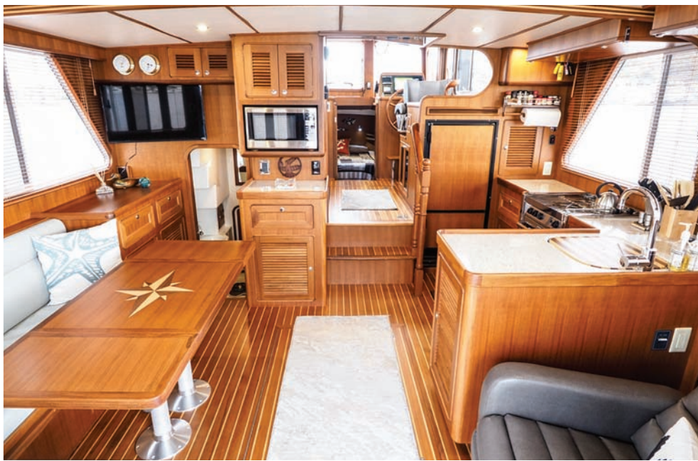
The standard layout of the salon and galley area is as depicted in this photo. Our test boat was a near mirror image of this, with the salon to starboard and the galley to port. The refrigerator/freezer gets a little smaller in the mirror layout, but other than that, nothing is lost.
